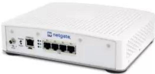
The Netgate 4200 is ideal for pro-home, small/medium businesses, branch and edge deployments that require flexible port configurations to support 1 to 2.5 Gbps WAN capabilities across four discrete, unswitched 2.5 Gbps RJ-45 ethernet LAN ports - all in a silent desktop form factor.
